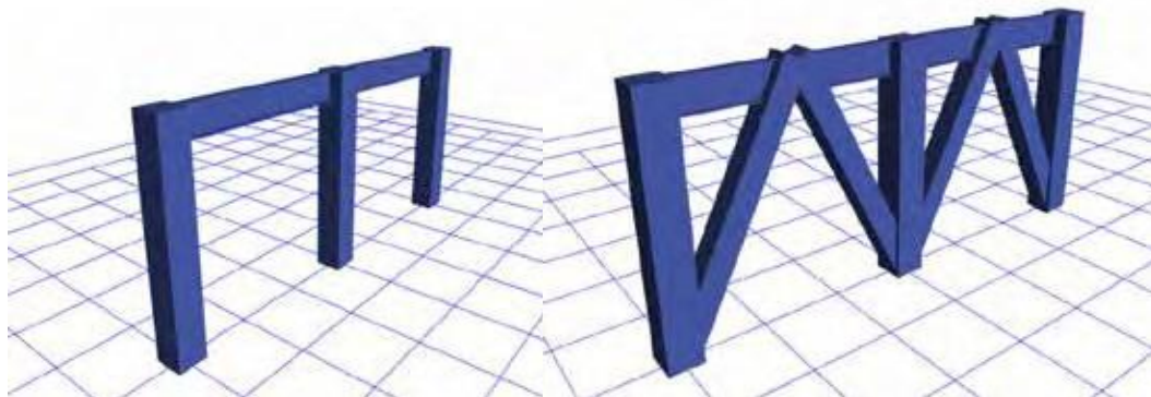
(a) Portal frame (b) braced frame Fig. 4: three-dimensional view of the frame
