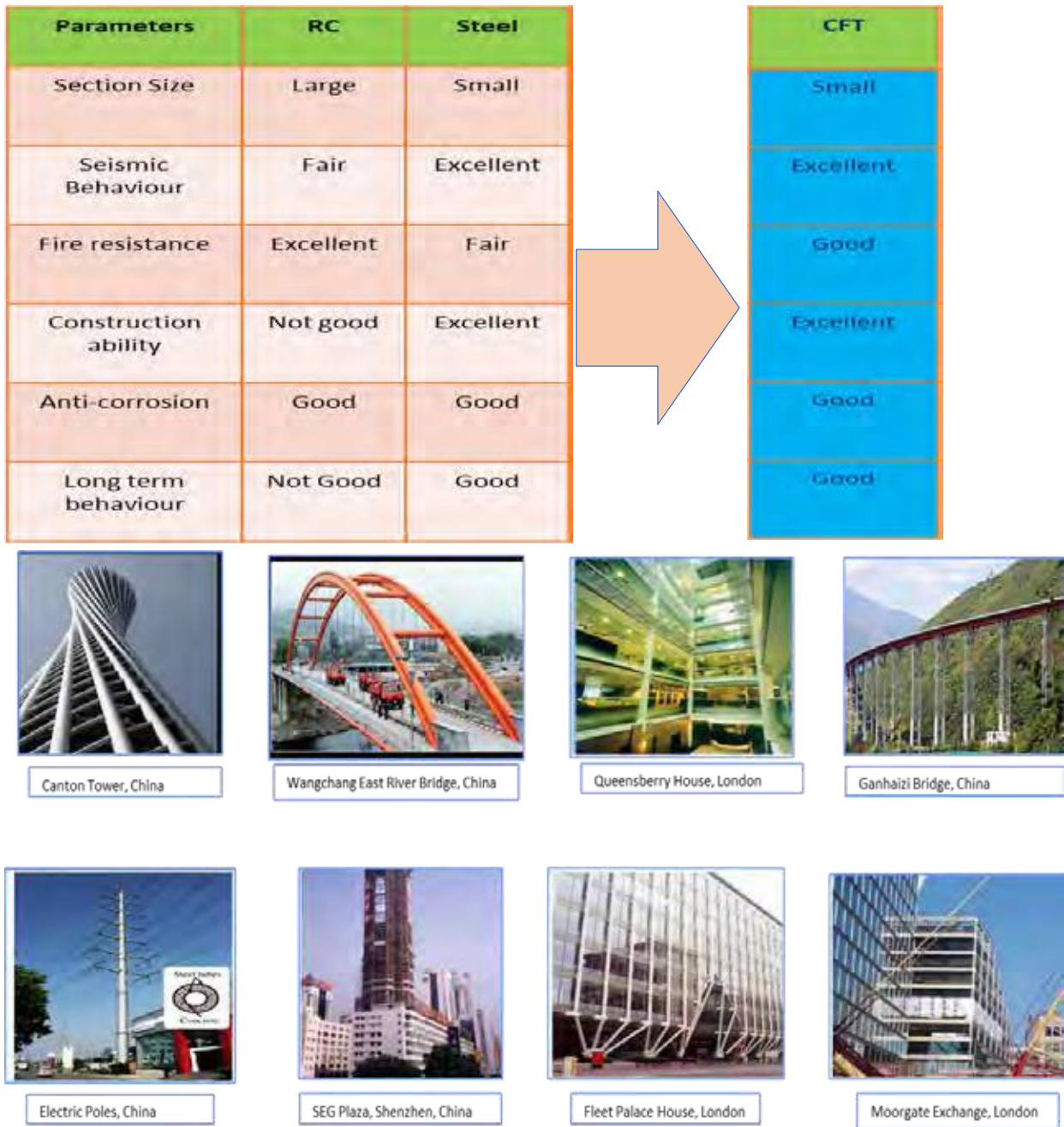
Fig.7: Some Major CFT Projects Outside India
