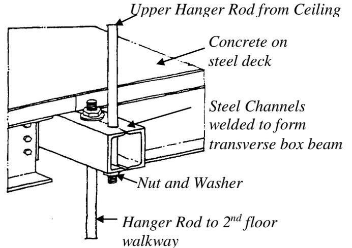
**Fig. 5(b): Hyatt Regency Hanger Details As-Built**
