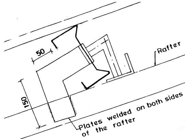
*Fig.17: Solution adopted to hold the purlin in place*
