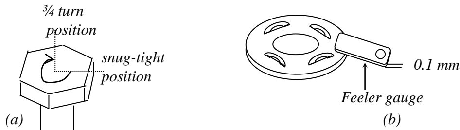
Fig. 5 Tightening of HSFG bolts
